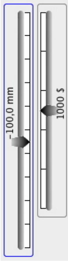
Figure 15: Container **CSliderV**. You can set the value indicator (1000 \$ ou 100,0 mm) to the left (kGradLeft) or to the right (kGradRight) the container's cursor..
